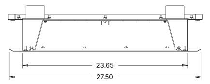
The part of the housing sleeve that penetrates the ceiling is nominally 23.65" x 23.65". The suggested 24" x 24" cutout provides 0.35" total clearance for each dimension.
